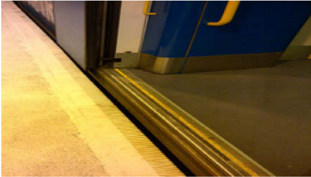
Figure 10. Platform Gap Fillers
